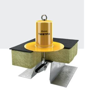
It is designed for mounting on flat roofs with thermal insulation. It is installed through the roof insulation using a special anchor for structural elements such as trapezoidal sheet, reinforced concrete, hollow core slabs.
