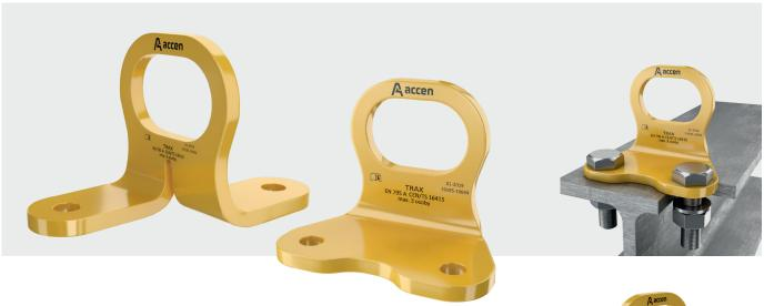
Anchoring point Duo/Duplo ST is an anchoring device fixed to steel sheets of minimum thickness 5 mm, intended for attaching devices of individual protection to prevent from falling from a height for maximum three persons at the same time.
