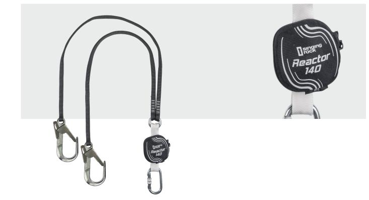
V-shaped belt fall protection lanyard, with integrated energy absorber (EN355 + EN 362), designed to move on the railing, in fixed belaying systems, between anchor points or on ladders. Ideal for employees moving on structures, ladders and poles. The low weight and practical shape do not limit the user at work, the lanyard is designed to safely stop the fall of a person weighing 140 kg (including equipment).
